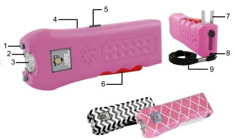
**Important:** The Disable Pin (attached to the wrist strap) must be inserted into the bottom of the unit in order for the stun to operate. The alarm and light will both function without the Safety Pin inserted.
