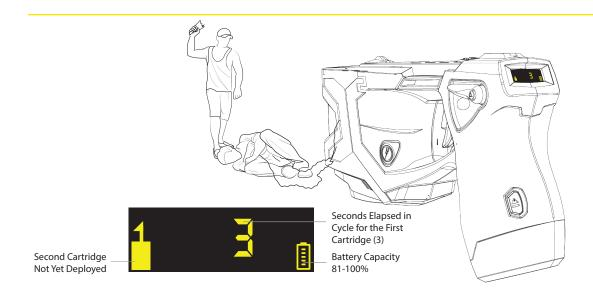
The X2 CEW energizes the first cartridge. Releasing the trigger automatically selects the next cartridge while the first cartridge is deploying.
