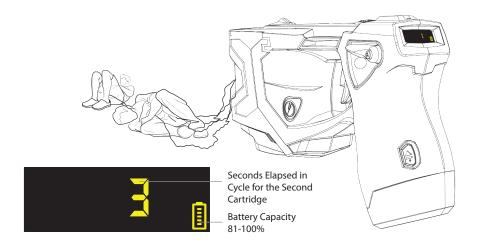
When both the first and second cartridges are energized each of the two firing bays will run for approximately five seconds on its own counter. If the second cartridge is deployed while the first cartridge is still energized, the first cartridge's cycle will end before the second cartridge's cycle ends. Therefore, to energize both cartridge bays, press the ARC switch. If the ARC switch is held down after the second cartridge's cycle ends, both cartridge bays will continue to cycle.
