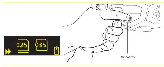
Pressing and releasing the ARC switch quickly selects the second cartridge.
