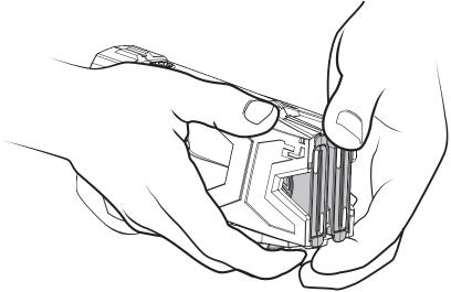
6 By loading from the right cartridge bay to the left bay (or left to right if the right hand is used), it is less likely the operator will place fingers in front of the blast doors of loaded cartridges.
