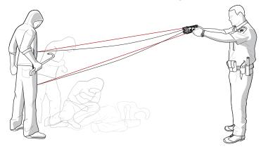
TASER technology is designed to use electrical impulses similar to those in your body's nervous system to cause stimulation of the sensory and motor nerves. Neuro Muscular Incapacitation (NMI) occurs when a CEW is able to cause involuntary stimulation of both the sensory nerves and the motor nerves. It is not dependent on pain and can be effective on subjects with a high level of pain tolerance.
