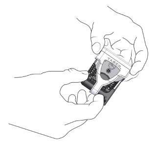
4 Push against this tab while pulling the cartridge out. You might consider pushing on the cartridge with your thumbs and holding the cover with your fingers. There should be an audible click when the cover releases the cartridge.
