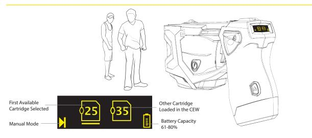
1 Pull the trigger switch to deploy the first cartridge.
