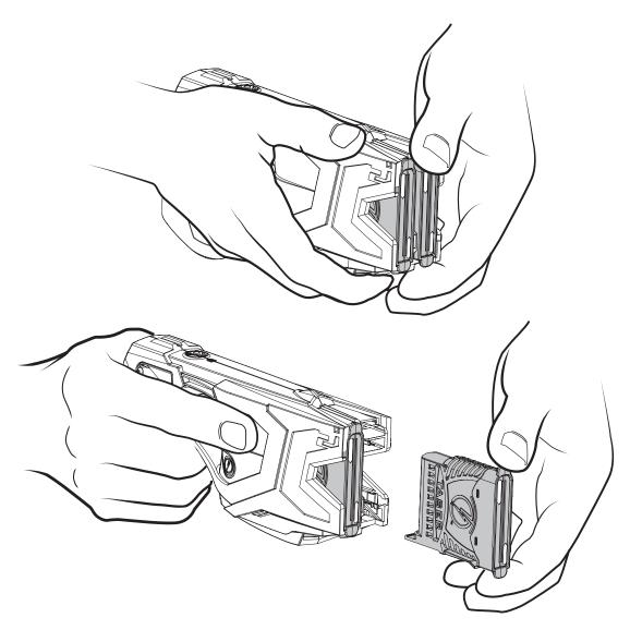
The Smart Cartridges can be reloaded independently. That is, if one of the two cartridges has been expended, you can replace the expended cartridge with a new one. You do not have to wait until both cartridges have been expended before reloading.
