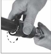
Do not pull the lower section past the "STOP HERE" warning on the handle shaft. If this does happen, re-align according to the diagrams at the right.
